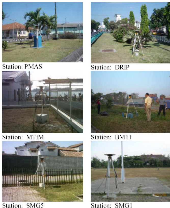
Figure 9. Example of GPS stations for monitoring land subsidence in Semarang.
